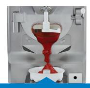
Thanks to the **spacer**, which can be mounted at any time, it is possible to reduce the door opening, thus facilitating the extraction of the Crystal product and the washing of the machine.
