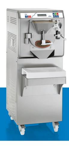
Performance and Quality Mix, heat and freeze in the same cylinder. Hard-O-Tronic technology: automatic consistency control to determine when the product is complete. POM Beater resists extreme hot and cold temperatures and includes auto-adjusting scrapers for complete extraction. Post Cooling ensures frozen dessert is cold upon extraction. Includes two separate beaters for Ice Cream and Gelato production.
